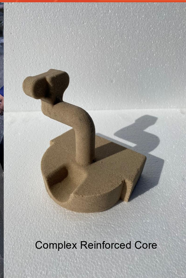
No-Bake Mold with a 3D-Printed Core
