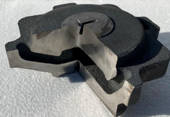
Condensate Drain Body Ductile Iron Casting, 1.27 kg
