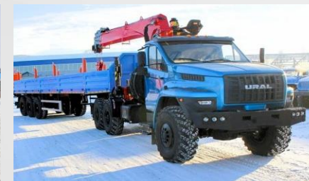
Tractor Unit with Crane Manipulator
